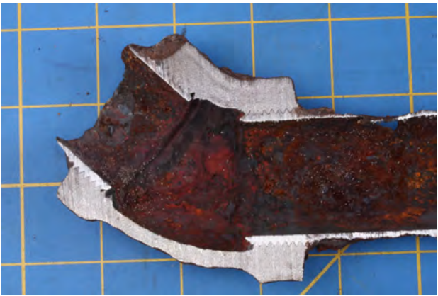
Figures 6. Sample 113950 and 113951 Figures 5A, documents the samples as recieved. Figures 6B,C,D, and E reveal the exterior and interior of the sample 113951 after sectioning as well as before and after media blast cleaning.
